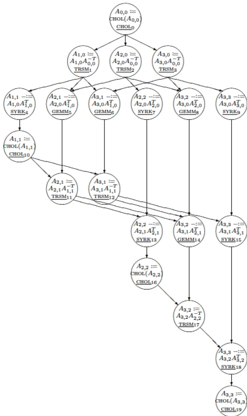
Figure 6.30: Graph of task dependencies in a 4 \times 4 Cholesky factorization
