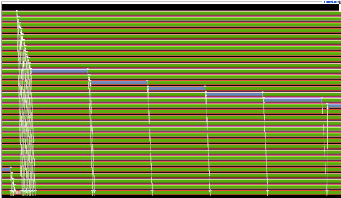
Figure 49.2: Trace of a serial Mandelbrot calculation
