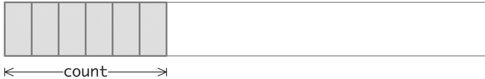
Figure 6.1: A contiguous datatype is built up out of elements of a constituent type
